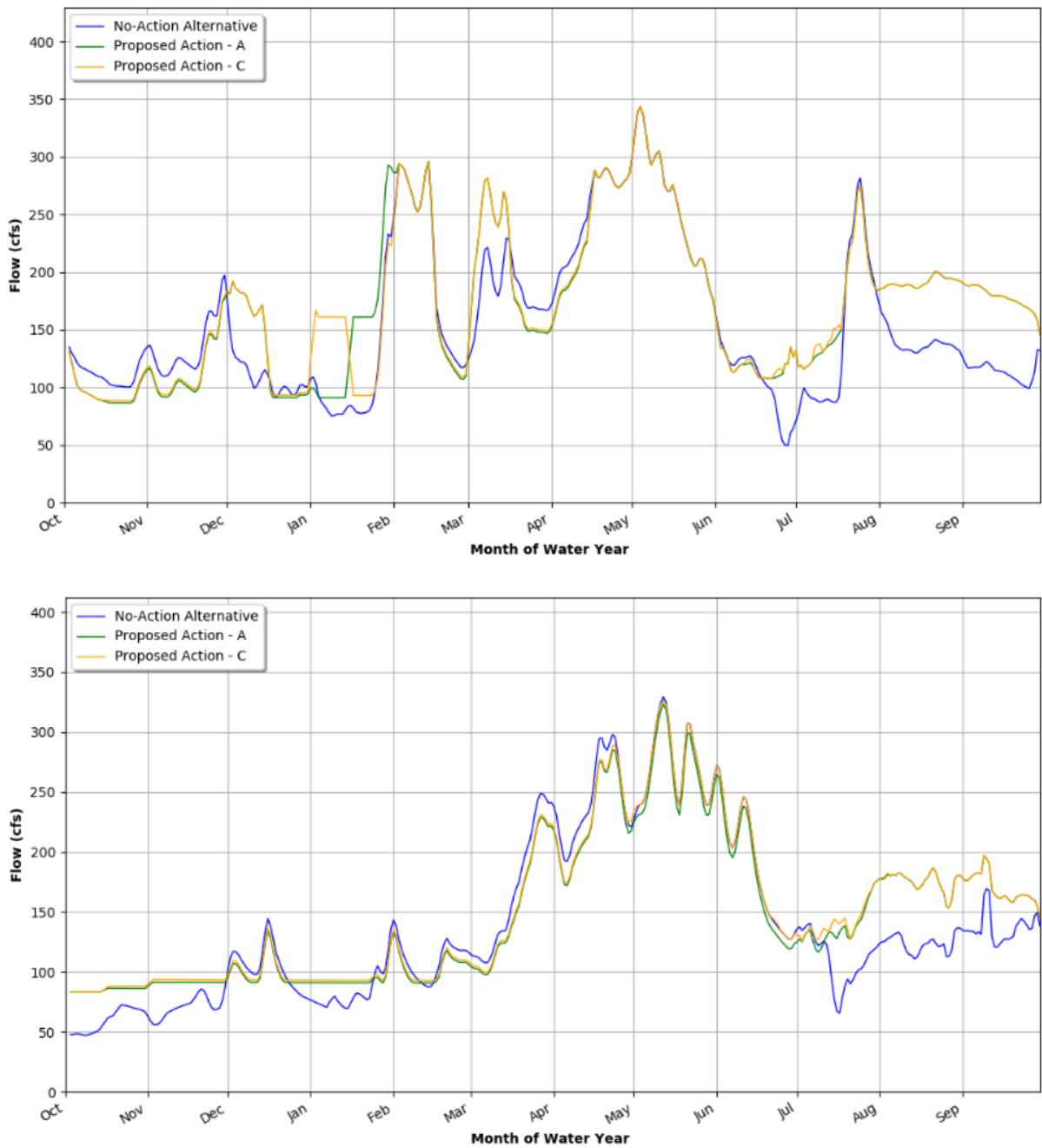
Figure 41. Modeled Flows for the Little Deschutes River at the LAPO Gauge under the Proposed Action Years 1–7 (A) and Years 13–30 (C) in Normal (upper) and Dry (lower) Years Compared to the No-Action Alternative
