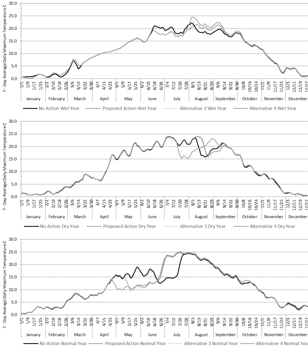
Figure 10. Annual Water Temperature Predictions (7-Day Average Daily Maximum) for the Crooked River (CAPO node) based on the 2019 RiverWare Model for a Wet (top), Dry (middle), and Normal (bottom) Year under the No-Action Alternative, Proposed Action, Alternative 3, and Alternative 4
